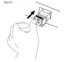
2. Link with fiber cable and Cat.x patch cord. Please make sure be right mode fiber cable, right Cat.x class.
